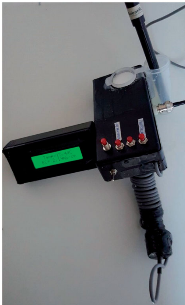
Figure 1. The final prototype of the portable device for measuring conductivity in Sarda sheep milk.
