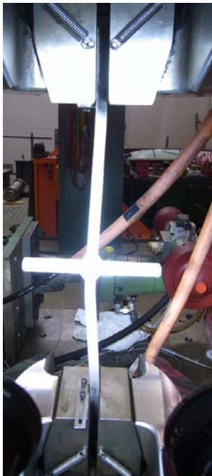
Figure 17: Deformed shape of specimen at F_{min} .
