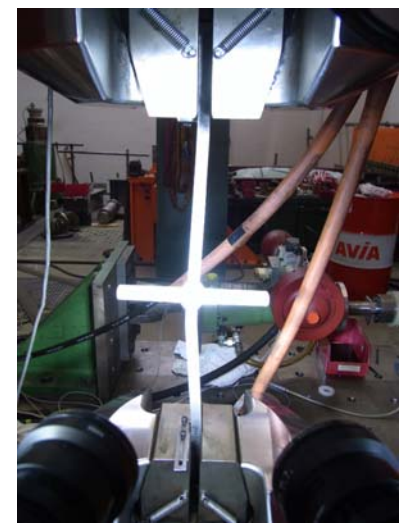
Figure 9: Deformed specimen at F_{min} .
