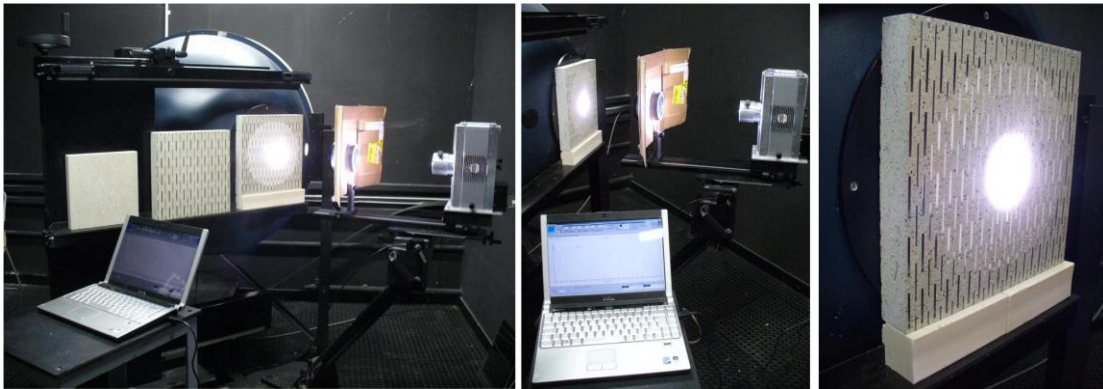
Fig. 3. (a,b)View of the optical bench including: the light source, the integrating sphere, the sample holder for the transmittance mode. (c) shows the experimental facility in the transmittance measurement mode. The spectral transmittance was performed on the selected samples
