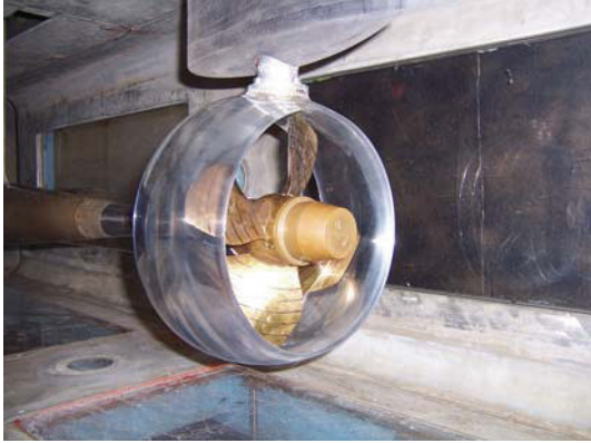
FIGURE 12: Measurement setup at cavitation tunnel.
