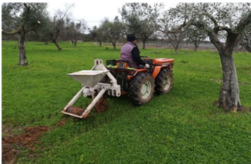
Figure 1. Furrower coupled with a distributor of the granulated Micosat F ®1 under Ogliarola di Lecce olive trees.
