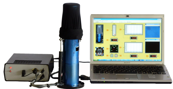
Figure 1: The system FYD: starting from the left side, it is possible to see the electronic box, which contains the motor driver and the DAQ card, the FYD prototype and a computer to control the system.
