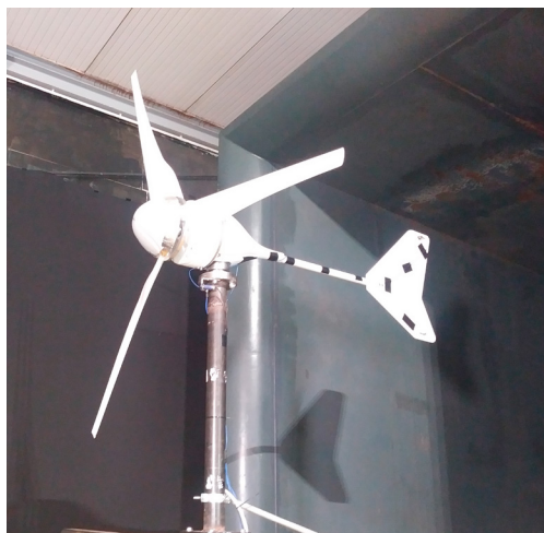
Fig. 2: The test case HAWT in the wind tunnel.
