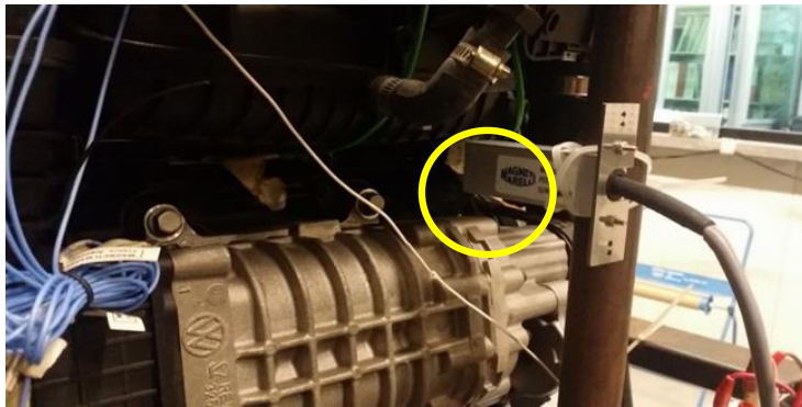
Fig. 1 Positioning of the Smart Acoustic Sensor.
