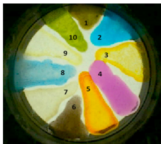
Figure 1. Image acquired by the camera of the artificial epithelium. Sensitive indicators are labelled according to the following list: 1: FeTPP 2: SiPC, 3: Methyl orange, 4: ZnTPP, 5: Bromocresol purple, 6: Biladiene, 7: TPC, 8: Nile, 9: Red Cresol, 10: MnTPP.
