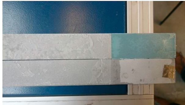
Fig. 6 - Portion of the fracture surface of the N01 nanomodified specimen
