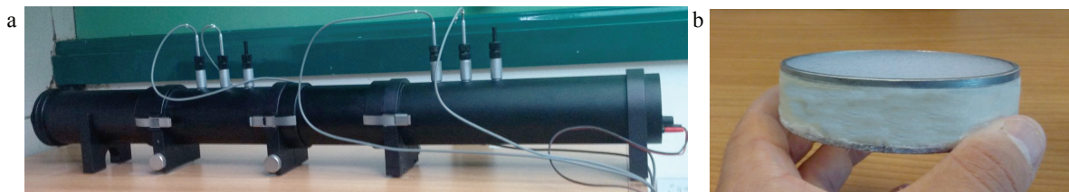
Fig. 2. (a) Impedance tube configuration for the transmission loss measurement; (b) aerogel in the sample port.
