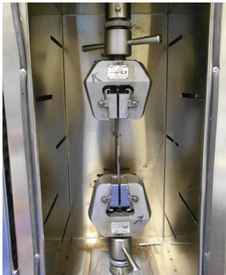
Fig. 2. Climate chamber used for high temperature tests.
