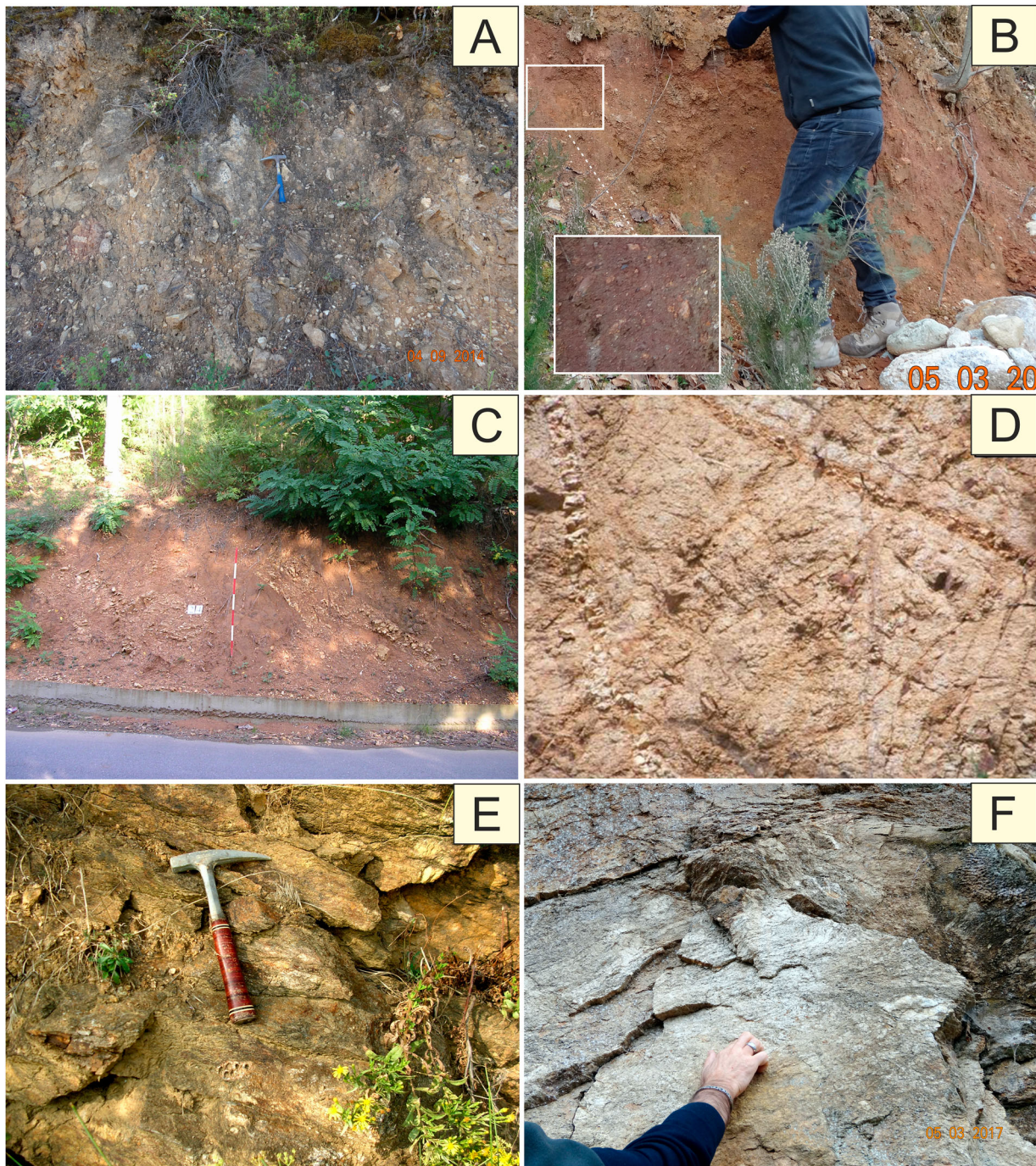
Figure 4. Examples of different classes of weathering in the gneissic rocks outcropping in the study area: (A) slope debris deposits (class VI); (B) colluvial soils (class VI); (C) residual soils (class VI); (D) completely weathered rock (class V); (E) highly weathered rock (class IV); (F) moderately weathered rock (class III).
