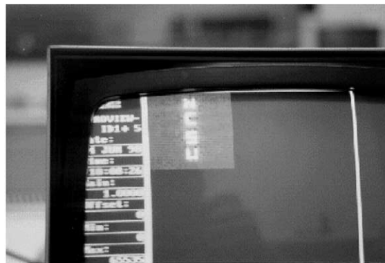
Fig. 53. Demonstration of a visible-blind UV image from a III-V nitride-based photo-diode array. The image from the FPA was recorded at NVL on July 28, 1999. (Courtesy of Prof. J. Schetzina).
