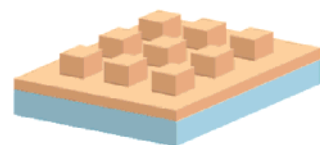
Figure 1. Schematic diagram of the RT-NIL process for the realization of 1D and 2D PhC-like patterns (features not in scale).
