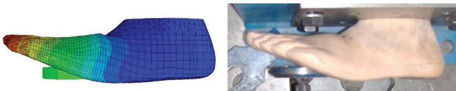
Fig. 6. Comparison between experimental and numerical displacements, for the foot component and toe-off loading condition (II) – scale 1:1.
