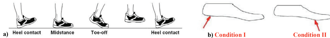
Fig. 2. Schematization of the stance for the normal walk (a) and related interpretation of the ISO 10328 standard (b).
