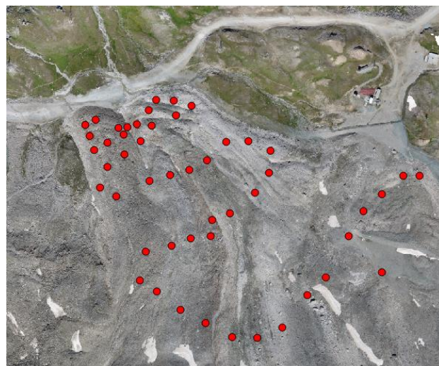
Figure 3: Localization of the 48 GNSS measured points.
