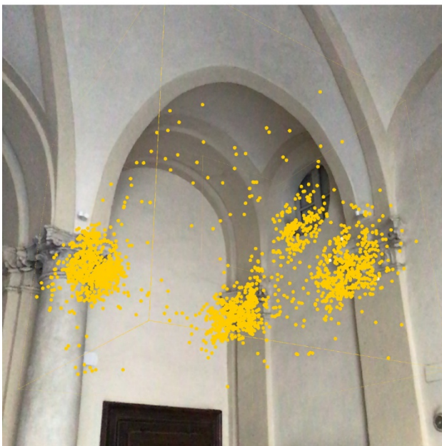
Figure 5: Screenshot of the scanner app: test of the larger bounding boxes for the scanning of target objects in the atria of Palazzo Carignano and Palazzo Cigliano
