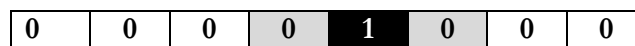
Figure 16: The simplest one-dimension CA grid. Each cell (say, that highlighted in black) has a state (say, 1) and neighborhoods (in the simplest case, the cell on the left and that on the right).
