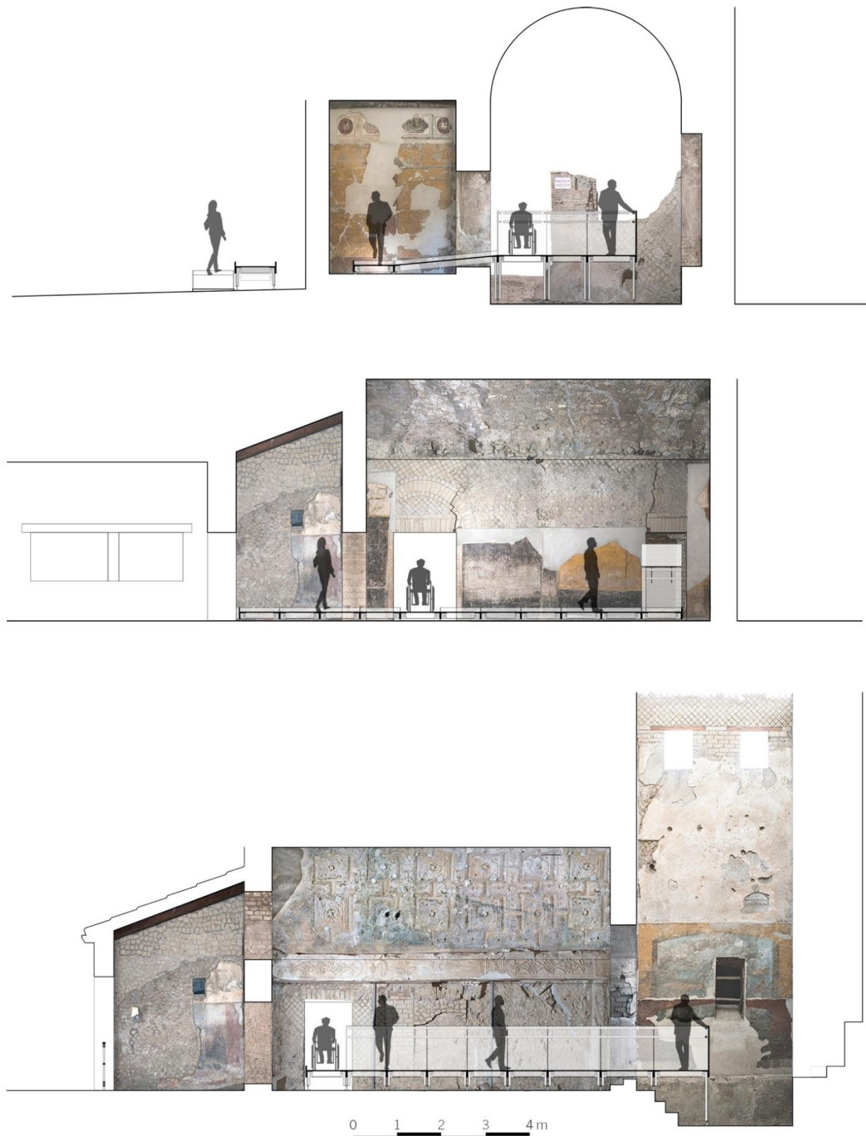
Figures 7, 8 and 9. Internal sections of the project for an improved fruition of the Suburban Thermal Baths in Pompeii, with the walkway in structural glass. From the top: natatio , apodyterium, frigidarium. (The research “Pompeii becomes accessible: a study of the accessibility to Pompeii archeological site through the entrance of the suburban Thermal Baths and the connection with the Antiquarium” was conducted by professors and scholars of the University of Naples Federico II: Renata Picone, Pasquale Miano, Paolo Giardiello, Gianpiero Lignola, Laura Bellia. Giovani studiosi: Stefano Belliazzi, Serena Borea, Luigi Cappelli, Giovanna Ceniccola; Mariapia Coccia, Ionio Conca, Sabrina Coppola, Francesca Coppolino, Giovanni Fabbrocino, Giuseppe Feola, Antonio Izzo, Antonella Lopardo, Fabiana Porreca, Giancarlo Ramaglia, Renato Rosa, Giovanna Russo Krauss, Viviana Saitto, Angela Spinelli, Antonio Stefanelli, Luigi Veronese. (Sections design by Antonio Stefanelli, 2018).
