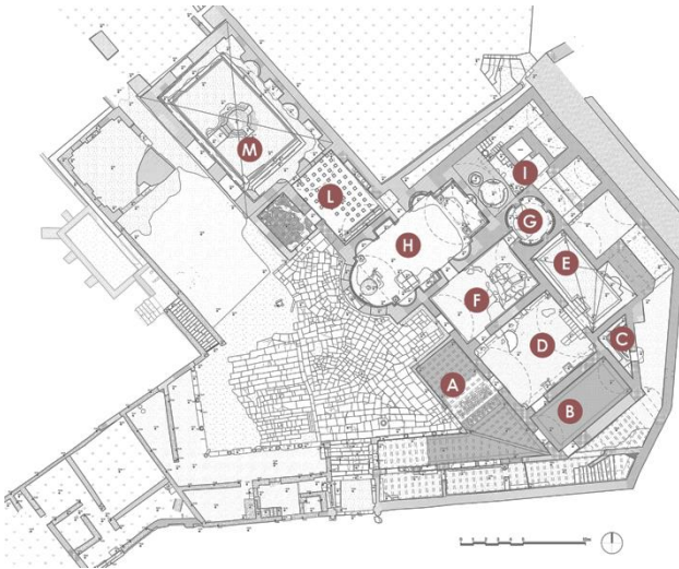
Figure 10. Planimetry of the Suburban Thermal Baths with the indication of the functions of the rooms: A. Entrance lock room, B. Apodyterium; C. Latrinae; D. Frigidarium; E. Cold Natatio; F. Tepidarium; G. Laconicum; H. Calidarium; I. Boilers; L. 'Warm' space; M. Warm Natatio. (Designed by: L. Cappelli).
