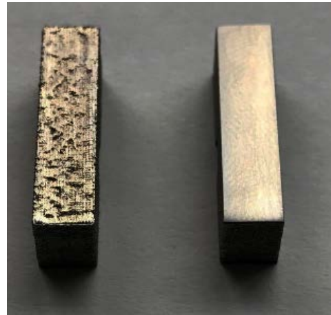
Fig. 3 As-built (left) and manual ground (right) surfaces of Type A specimens.
