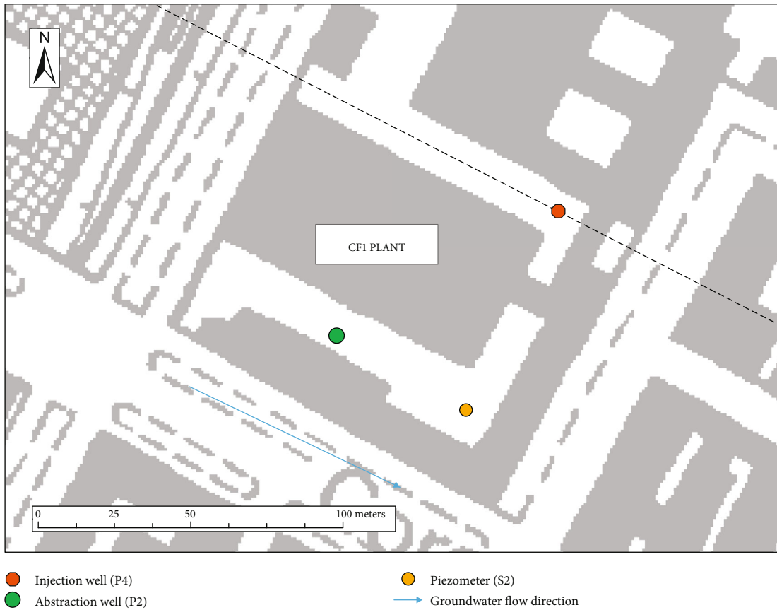
FIGURE 1: Politecnico CF1 plant GWHP system overview. P2: abstraction well, P4: reinjection well, S2: control piezometer. Dotted line indicates the direction of the cross-section line reported in Figure 3 [12].
