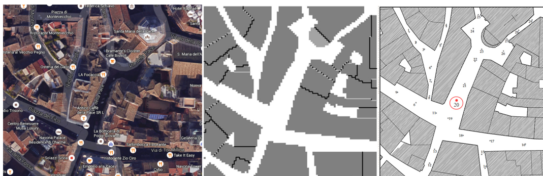
Fig. 1. Areal view of the urban portion selected for the microclimate simulations and representation of the model through ENVI-met. On the right, the 30 points of simulation data collection are identified (in particular, point 20).
