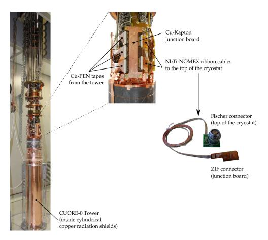
**Figure 14**. Photograph of the CUORE-0 tower attached to the dilution refrigerator, before the installation of the thermal radiation shields. Right: A zoom of a Cu-Kapton junction board, which connects the Cu-PEN cable to the NbTi-NOMEX cables which run up to the top of the cryostat.
