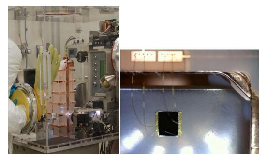
**Figure 12**. Left: The assembly workstation during the bonding operations. The bonding machine is on the right of the picture. Right: Detail of the bonding connection of a NTD thermometer. The gold pads of the thermistor are connected to the copper pads of the Cu-PEN cable through gold wires.
