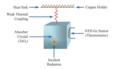
**Figure 1**. Schematic of a bolometric detector. A CUORE bolometer consists of an absorber connected to a heat sink through a weak thermal link, and read out by a temperature sensor attached to the absorber.
