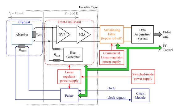
Figure 16. CUORE-0 electronics block diagram.
