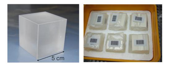
**Figure 3**. Left: A TeO<sub>2</sub> CUORE crystal. Right: Six TeO<sub>2</sub> crystals packed for transportation and storage: the crystals are triple vacuum-packed in plastic bags and they are stored in a vacuum packed box.
