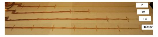
Figure 7. The four types of CUORE-0 Cu-PEN tapes. The picture shows the bottom  $\sim$ 80 cm of the tapes that were located on the sides of the tower.
