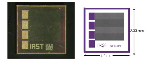
Figure 5. Left: Photograph of a CUORE-0 silicon heater. Right: Drawing of the heater geometry.
