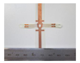
**Figure 8**. Detailed view of copper pads onto which the gold wires were bonded. The width of each copper track is 0.2 mm with a pitch of 0.4 mm. The total width of the tape is 13.4 mm, with a 1.0-mm minimum margin on each side.
