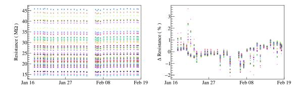
**Figure 23**. Left: Values of the CUORE-0 bolometer resistances at the working point measured daily over a period of one month in 2014. Right: Percentage variation of the same resistance values over the same time period. In both plots different marker colors and styles identify different bolometers.
