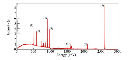
**Figure 24.** CUORE-0 calibration spectrum. The peaks are identified as  $\gamma$  lines from the decay of nuclei in the <sup>232</sup>Th decay chain: (1) 511 keV (e<sup>+</sup>e<sup>-</sup> annihilation), (2) 583 keV (<sup>208</sup>Tl), (3) 911 keV (<sup>228</sup>Ac), (4) 965 keV and 969 keV (<sup>228</sup>Ac), (5) 1588 keV (<sup>228</sup>Ac), (6) 2104 keV (<sup>208</sup>Tl with single 511 keV escape), (7) 2615 keV (<sup>208</sup>Tl).
