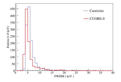
**Figure 25**. Comparison of the distribution of the energy resolutions (FWHM) measured in calibration for Cuoricino (blue dashed line) and CUORE-0 (red line).
