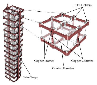
**Figure 2**. Left: A rendering of the CUORE-0 tower, including the wire trays for signal connection. Right: A single CUORE-0 detector floor, in which the  $TeO_2$  crystals, PTFE holders, and copper frames and columns are indicated. The copper frames are shared between adjacent floors.
