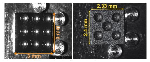
**Figure 10**. Glue-spot matrices deposited on a thermistor (left) and a heater (right) using the CUORE gluing workstation.
