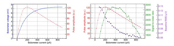
**Figure 21**. Detector characterization curves. Left: I-V curve (blue solid) and pulse amplitude curve (red dashed). Right: The same pulse amplitude curve (red dashed) with the baseline RMS curve (purple dotted) and their ratio (green solid).
