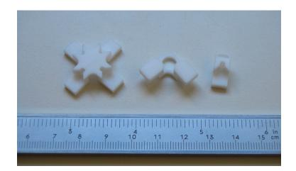
Figure 6. The three types of PTFE holders used for the tower construction.
