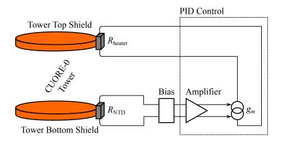
Figure 17. Temperature stabilization set-up of the CUORE-0 tower.
