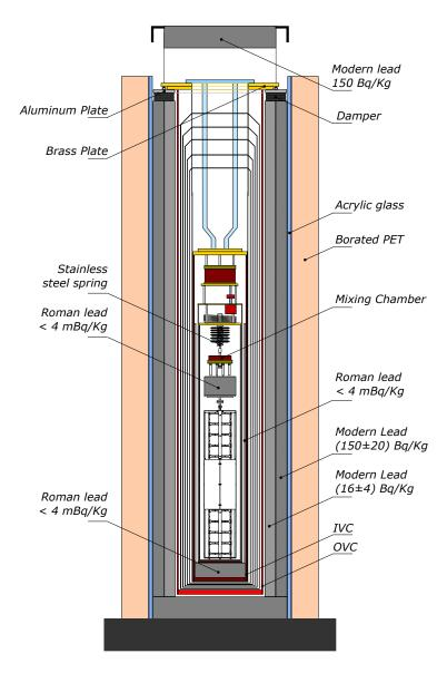
**Figure 15.** Sketch of the CUORE-0 cryostat and shielding (not to scale). The indicated activities refer to decays of <sup>210</sup>Pb.
