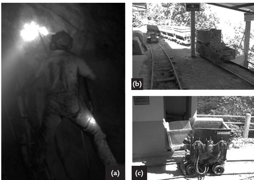
Figure 1 (a) Operator handling the manual pneumatic drill; (b) Hauling wagons (back) and electric locomotors (front); (c) Pneumatic loader. In b/w for a better resolution of the pictures taken underground
