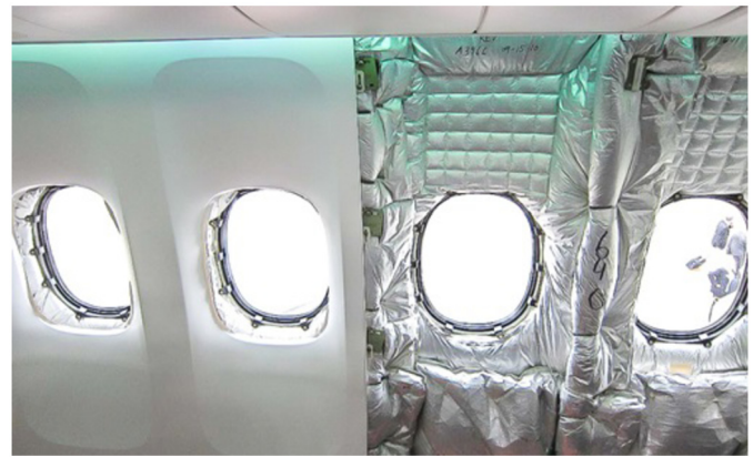
Fig. 5. Typical sidewall treatment of a large passenger transport aircraft.
