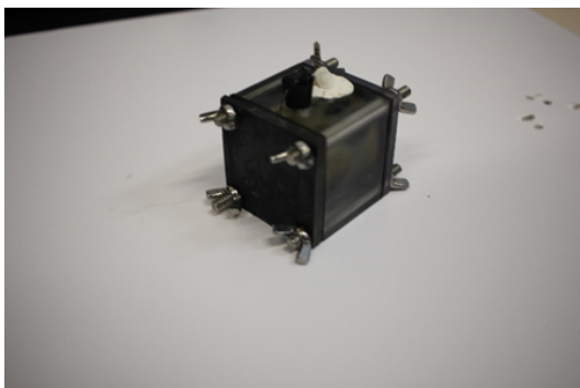
Fig.1a BC-MFC cathode on a cubic shape cell
