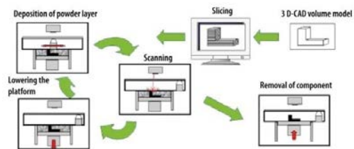
Figure 6 Powder Bed Machines, courtesy of Fraunhofer IFAM
