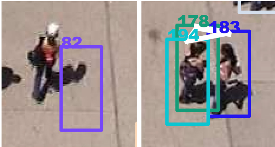
Fig. 9. Tracker errors. Some of the tracker errors are caused by a wrong initialization. In the left figure, the shadow is detected instead of the person. Furthermore, the shadow moves indeed like a human, and this makes it harder for the inference to infer that there is a failure. The right figure shows another mistake. This time is the bag that is being recognized as a person and is also being assigned the same group as the other two subjects.
