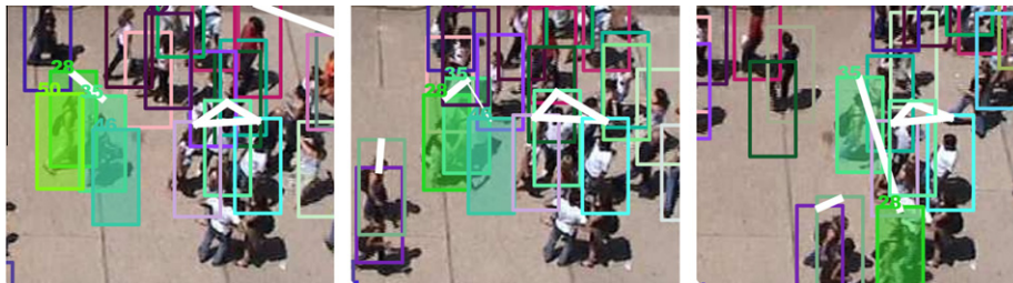
Fig. 10. Tracker failure detection. Sometimes, the initialization or the tracker itself lead to a wrong estimate. The leftmost figure shows such a case, where for the two subjects with ID 28 and 35, there is another pair of wrong estimates, namely 50 and 46. The tracks of interest are represented with a shaded bounding box. The tracker finds out that the estimates are wrong in the following frames. This happens because the wrong tracks violate the avoidance behaviors, since they overlap with other tracks and lack of a strong observation support. We show frames, from left to right 1175, 1200 and 1250.
