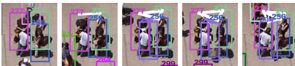
Fig. 8. Group formation. The thickness of the white line is proportional to the estimated probability of the two subjects being in the same group. The frames being shown are, from left to right, 4000, 4100, 4300, 4320 and 4350.
