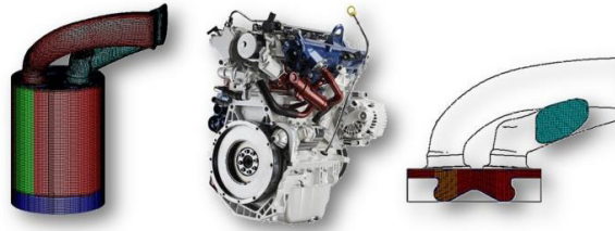
Fig.5 Common Rail Diesel Engine and Fully 3D computational mesh used
