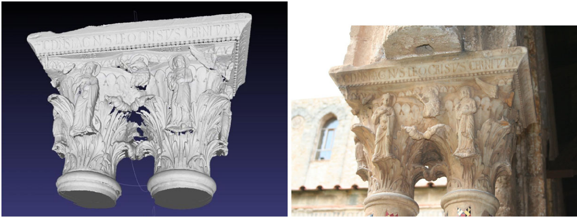
Fig. 1 A rendering of an uncomplete model, where part of the geometry could not be acquired with laser scanner (missing regions are easily detectable especially in the bottom side of the capital) and a photograph of the real artifact
