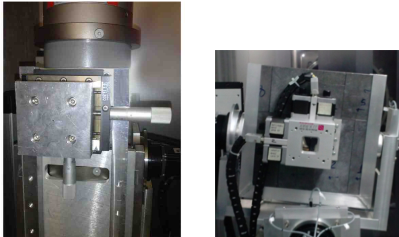
Figure 2. The X-ray tube ( left ) and the Tungsten collimator ( Right ).
