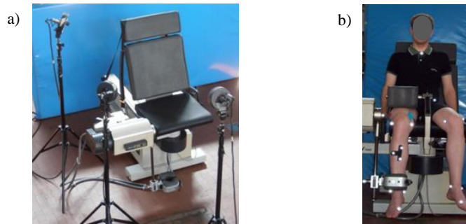
Fig.1. a) Technogym REV 7000 and BTS optoelectronic system (only three cameras are shown); b) Markers, electrodes and testing conditions.
