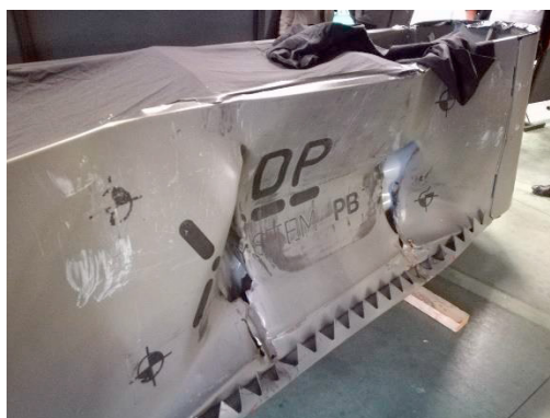
Fig. 8. Anti-terror barrier after the experimental test.
