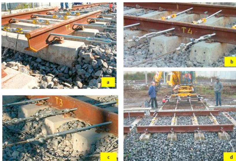
Fig. 6. Lateral resistance layouts for track panels: (a) without ballast crib; (b) with base contribution only; (c) without shoulder; (d) with ballast everywhere (De Iorio et al. (2018)).
