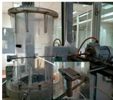
Fig. 2. Plexiglas reactor used for the FBM experiments, with a detailed image of the samples clamping system placed inside (abrasives not present).
