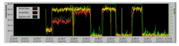
**Figure 1.16:** Beam intensity measured by the WCMTB01 on the BTF line (red trace), compared with the intensity at the end of the LINAC measured by WCMTM01 (yellow trace), and their ratio (green trace), during a typical operation cycle (no beam periods correspond to switches among electron and positron mode of the LINAC).
