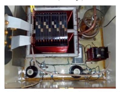
**Figure 3.4:** The klystron tank, hosting the pulse transformer and the capacitive divider 10,000:1 (for the measurement of the input klystron potential,  $V_k$ , on the top right of the picture).
