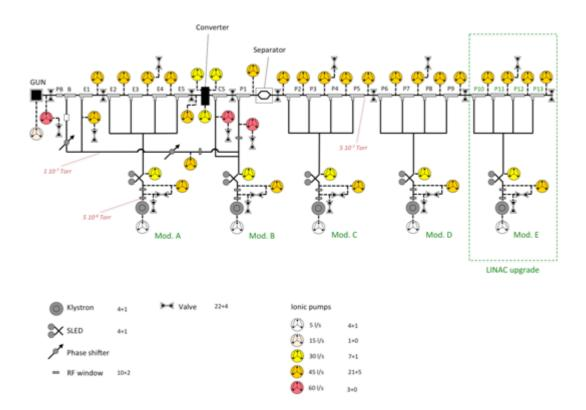
Figure 3.15: Extended LINAC vacuum system preliminary layout.
