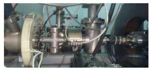
**Figure 1.6:** The effect of first focussing coil (in the middle of the picture) has to be compensated near the cathode by the bucking coil (on the left). On the right, the first of the 14 Helmholtz coils is visible.
