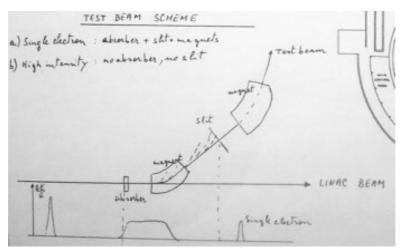
**Figure 1.8:** Original sketch of the beam-test facility line.
