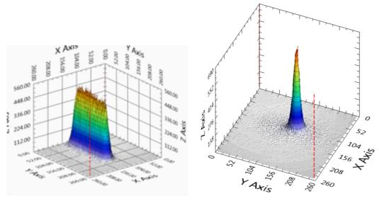
**Figure 1.21:** 450 MeV electrons imaged by Medipix Silicon pixel detector with SLTTB02 slits open at 2 mm (left) and 0.5 mm (right). The optimized beam on the right pane has a fairly Gaussian shape with  $\sigma_x \times \sigma_y = 0.5 \times 0.5 \text{ mm}^2$ .
