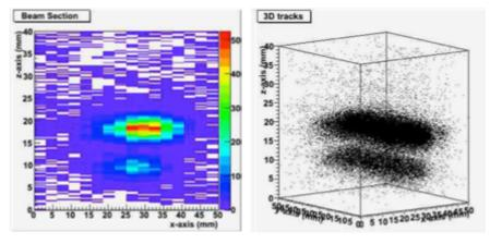
**Figure 1.18:** 477 MeV positrons split in two beam spots by channeling in a five-fold fan of planar crystals (*xz* and 3D view).
