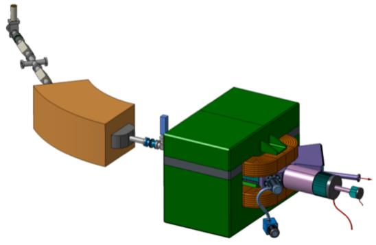
**Figure 2.7:** PADME setup sketch, installed downstream of the DHSTB02 last BTF dipole (orange): inside the poles of the large (green) analysing dipole a vacuum pipe with positron veto scintillating detectors is connected to the downstream vacuum decay volume, ending with the BGO crystal calorimeter. A central hole allows forward Bremsstrahlung background photons to hit a fast small angle calorimeter. The primary positron beam is swept away from the calorimeter by the same dipole field.
