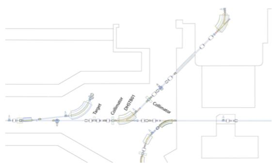
**Figure 1.10:** Layout of the original BTF beam attenuation and extraction system (until 2004) with the main elements (target, dipole, collimator) on the main injection line.
