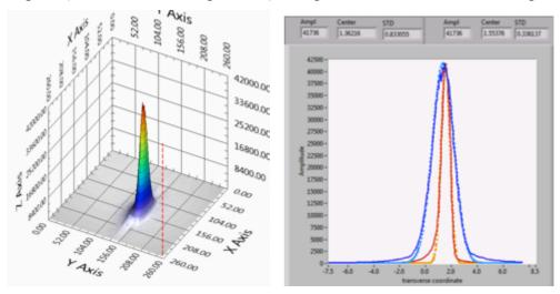
**Figure 1.23:** 450 MeV electrons imaged by Medipix Silicon pixel detector: an additional Tungsten collimator is placed downstream of the exit window, reducing the beam size in the horizontal coordinate (red histogram in right plot) to  $\sigma_x$ =340  $\mu$ m, leaving the vertical one (blue histogram in right plot) unchanged.
