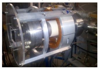
**Figure 1.15:** Main BTF exit (after the 45° bending of the DHSTB02 dipole) showing (from right to left): the pre-vacuum port and valve, the integrating current toroid around the ceramic gap in the beam pipe, the flange with the thin (0.5 mm Beryllium) window and relative Plexiglas protection.
