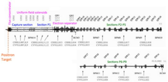
**Figure 1.7:** Scheme of the second part of the LINAC, downstream the positron converter.
