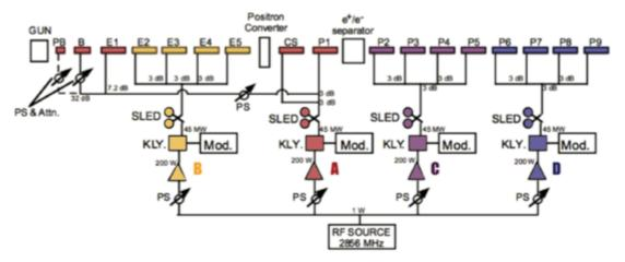
Figure 1.2: RF distribution scheme of the LINAC.
