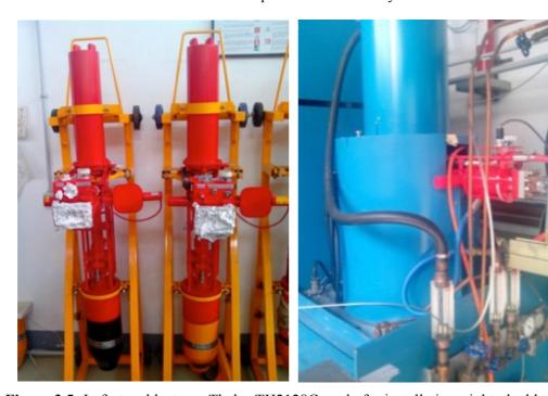
**Figure 3.5:** Left: two klystrons Thales TH2128C ready for installation; right: the klystron installed inside the cooling oil tank and surrounded by its focalizers.
