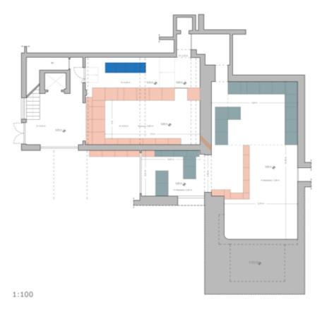
**Figure 3.20.a:** Proposed layout of the two new experimental areas, without moving the four DA $\Phi$ NE instrumentation racks and without modifying the access to the building.
