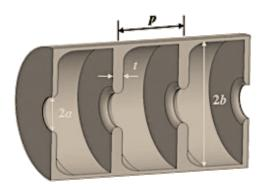
**Figure 3.9:** Scheme of the disk-loaded accelerating structure of radius *b* and cell length p; disks have thickness *t* and internal radius *a*.
