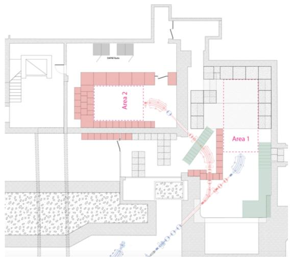
**Figure 3.19:** Proposed layout of the BTF beam-line, modified to have two lines, one in the existing experimental hall, and one serving the second area in the former control room.
