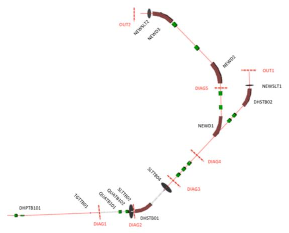
**Figure 3.22:** Graphical display of the G4-beamline simulation of the new beam-lines, showing the new elements and the detecting volumes (DIAG1 to DIAG5). The line coincides with the present line up to the DIAG3 position. The two final detecting volumes are OUT1 (BTF1 line, in the present area) and OUT2 (BTF2 line, in the new hall).
