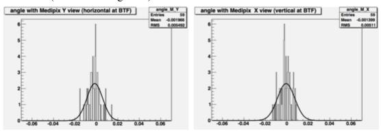
**Figure 1.25:** Angular divergence of 450 MeV electrons reconstructed by a couple of Medipix Silicon pixel detectors in the horizontal (left) and vertical (right) coordinate. In this plots the usual convention *x* for horizontal, *y* for vertical was exchanged.
