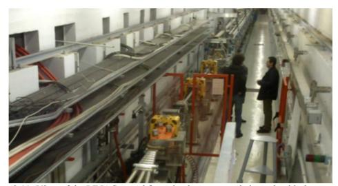
**Figure 3.11:** View of the LINAC tunnel from the three-way switch-yard, with the two pulsed magnets driving the beam towards the BTF line (3°, yellow dipole) and the spectrometer line (6°, orange dipole), towards the LINAC (top of the picture). In between, a  $\approx$ 15 m drift, with four quadrupoles (yellow). In the upper part of the picture, the passageways towards the parallel modulator tunnel for cables, pipes and waveguides, is visible.
