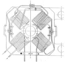
**Figure 3.13:** Two FODO wrap around quadrupoles are foreseen for each of the 3 m SLAC accelerating sections: picture of existing ones (left) and mechanical design (right).
