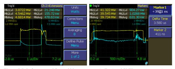
Figure 3.7: Left: measured forward klystron power (yellow) and SLED output power (cyan) for one of the four RF stations. Right: measured forward (yellow) close to the maximum klystron power  $\approx$ 41 MW, and reflected (cyan)  $\approx$ 1 MW.
