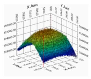
**Figure 2.9:** Spatial distribution, measured with Medipix detector over a  $1.45 \times 1.45 \text{ cm}^2$  sensitive area, of 50 MeV electrons,  $3.5 \times 10^3/\text{pulse}$ , during a test BTF irradiation run.
