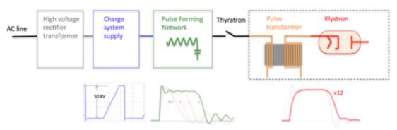
**Figure 3.2:** Logical scheme of the modulator, thyratron and pulse transformer supplying the klystron.
