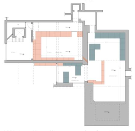
**Figure 3.20.b:** Proposed layout of the two new experimental areas, in the hypothesis of moving the four DA $\Phi$ NE instrumentation racks and with enlarged access to the building.
