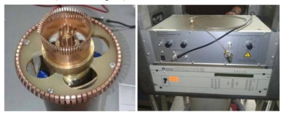
**Figure 1.3:** Electron gun cathode socket (left), and isolated high voltage station with new pulsing system (right).
