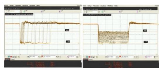
**Figure 1.4:** Rectangular waveform pulsing the electron gun, with variable length between 1.4 and 40 ns (left) and amplitude between 300 and 750 V (right).
