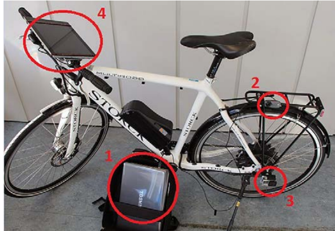
Fig.2 Data collection setting: 1) the laptop with software for acquisition of inertial data and the USB Bluetooth; 2) the webcam; 3) the high-speed camera; 4) the tablet
