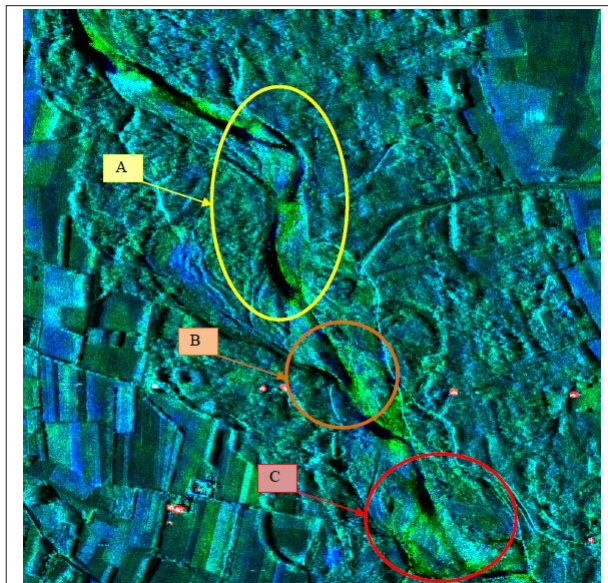
Figure 6 - Orco River, COSMO-SkyMed Level-1a product. Blue band: 24 June 2010 (reference image); Green band: 28 September 2010 (test image, low flow discharge); Red band: interferometric coherence. Circles marked with the letters A, B and C highlight planform changes.
