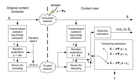
Fig. 2. Block diagram of the proposed tampering identification scheme
