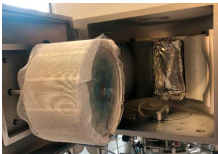
Fig. 2. Sputtering chamber and basket used for handling the pellets
