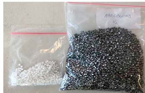
Fig. 8. Nano-particles silver coating of Arboblend V2 sample
