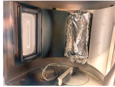
Fig. 3. Targets position and shutter inside the chamber
