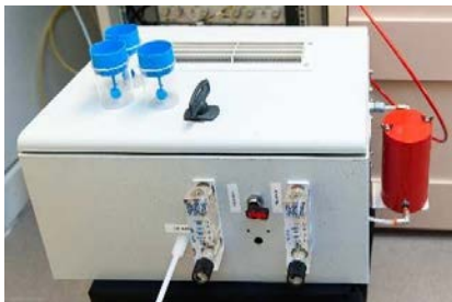
Fig. 1: the device A1 for CRC preventive screening through fecal exhalation analysis.
