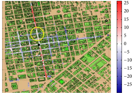
FIGURE 5: Map of the error [dB] for site A0000F8D. BS position is shown as a black dot.
