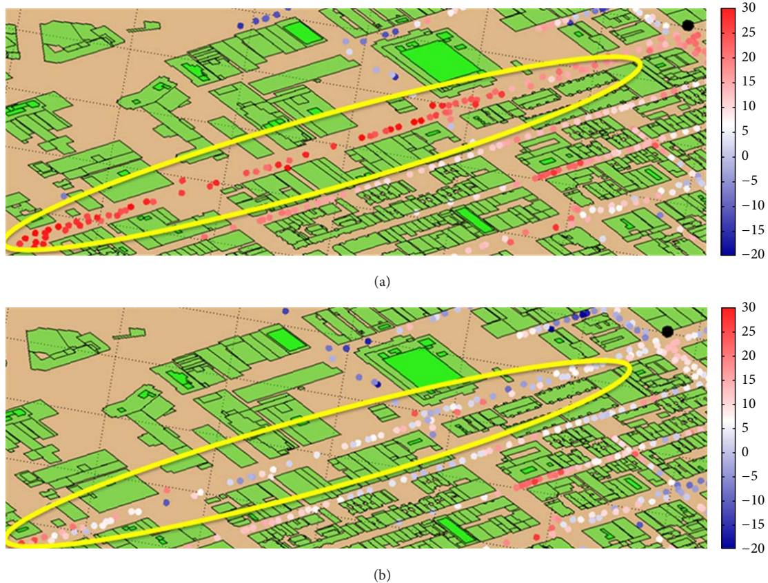
FIGURE 7: Impact of the ray selection method in urban street canyons: (a) error map [dB] obtained including rays with multiple reflections/diffractions; (b) error map obtained including only LOS ray in the street canyon [site A0000A49; BS position is shown as a black dot].
