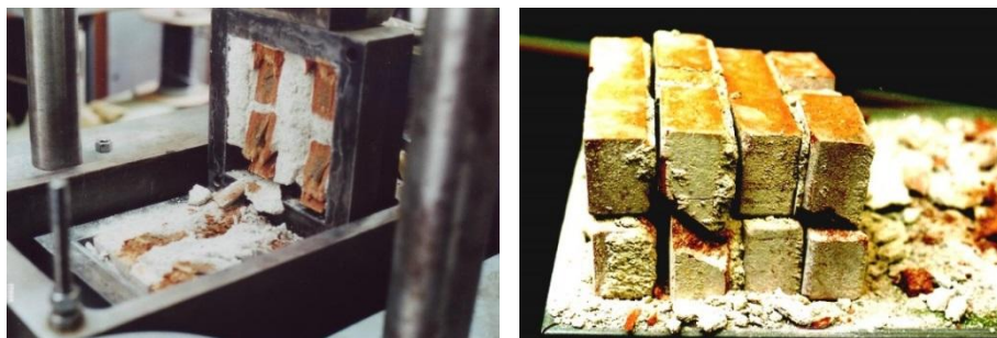
Figure 5: Masonry specimen in the shear box (left) and after the shear test (right).
