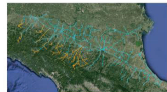
Figure 4: Lepida network with its wireless extensions (orange)
