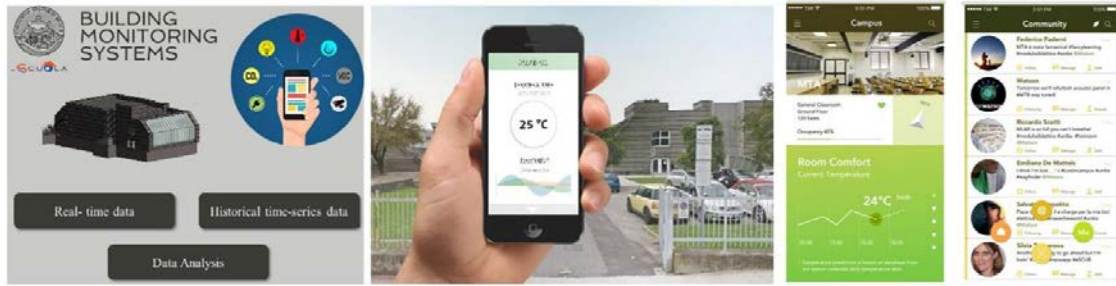
Fig. 4. The proposed interface of the web app and the mobile device layout in which the monitored data are displayed for the user awareness and feedback; the advanced idea is to introduce a community in which to implement the IoT Watson by IBM to perform sentiment analysis.
