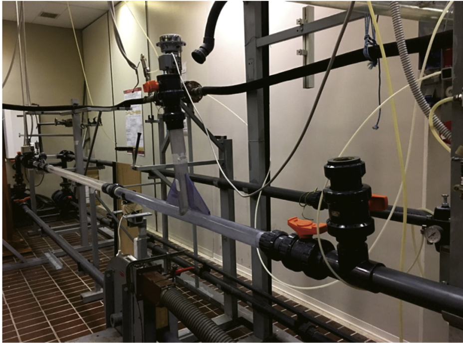
Fig. 2. Picture of air-water-sand flow loop at DIISM. Test section.
