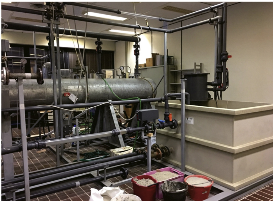
Fig. 3. Picture of air-water-sand flow loop at DIISM. Mixing tank and regulation valve.
