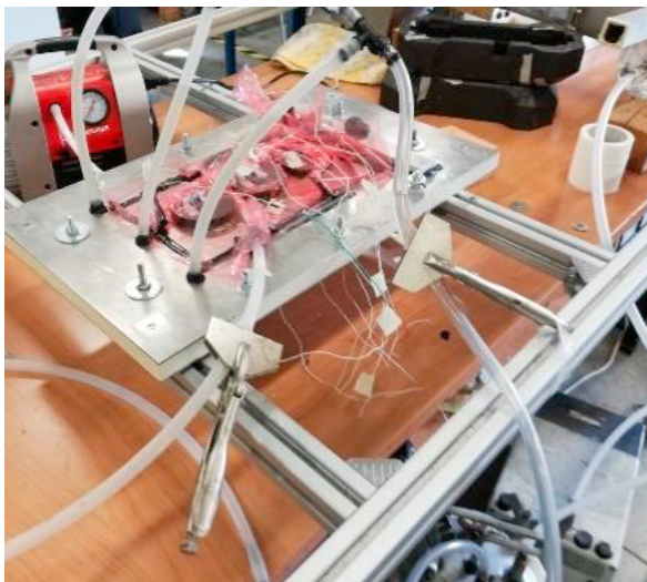
Fig. 2. Lab scale LCM line.
