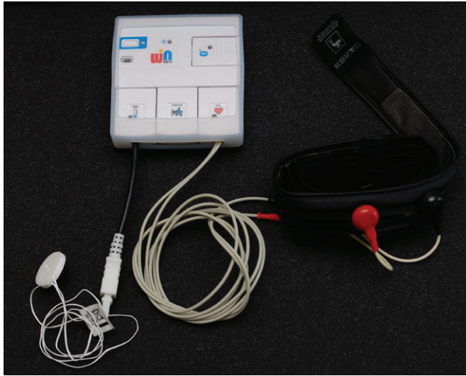
Fig. 1: WINPack1 with the connected sensor modules.
