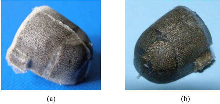
Fig. 1. Photo of iCub’s Fingertip sensors with dielectric made with: Soma Foama (a) and PDMS (b).
